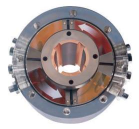
The rotary vane is a hydraulic powered actuator. Hydraulic force simultaneously forces both of the rotor's vanes away from the stationary shoes producing rotation and perfectly balanced torque output. Hydraulic input power is reversed for rotation in the opposite direction.
