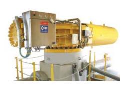
OLGAS QA is the quick-acting spring return hydraulic and electro-hydraulic actuators with high flow rate manifold and cylinder, integral quick exhaust valves, and end-of-stroke damper systems, designed by Biffi.
