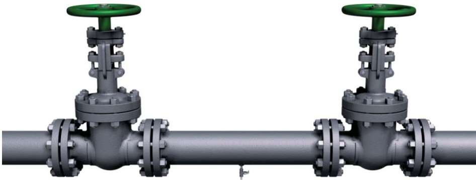
Historical double block-and-bleed system requiring the use of two valves and a spool piece. A bleed valve was used to drain the spool and verify seal integrity.
