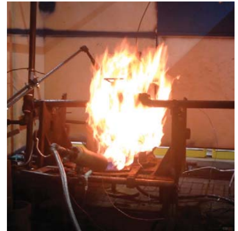
Fire test per API Spec 607 4th Edition.
