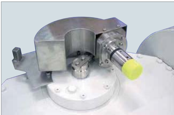
Position transducer assembly with electrical instrumentation connector.
