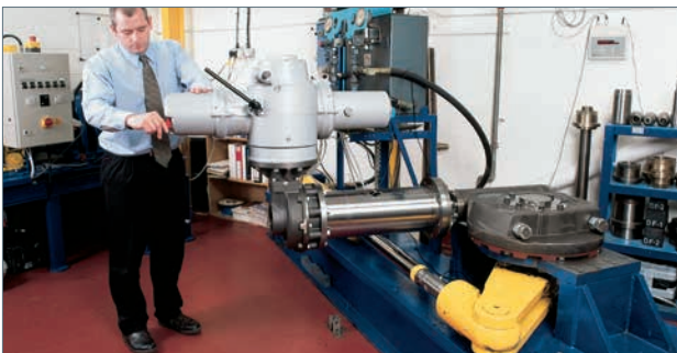
Endurance testing of prototype subsea gearbox.
