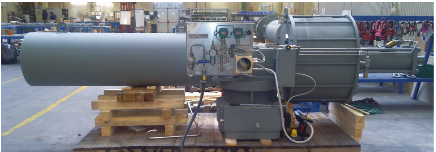
The Cameron LEDEEN® actuator mounted on a DYNATORQUE D-Stop partial-stroke test device.
