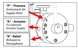
\*Note: Filter/regulator is recommended to ensure clean, dry air is supplied to block & bleed valve and actuator.
