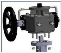
Gear operator is attached to valve by 4 or 8 bolts/studs (body tapped). A female drive is designed to accept a male valve stem or coupling w/ slip fit clearance.
