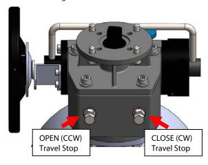
Two travel stops independently control the final stopping positions of the valve. The left stop sets the open position (full CCW rotation), and the right stop sets the close position (full CW rotation).
