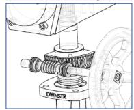
Valve, actuator, and segment gear are always permanently engaged when assembled. The clutch DOES NOT disconnect the actuator from the valve.
