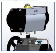
Actuator is attached to gear operator by 4 bolts/studs (body thru holes). A male drive on the gear operator is designed to insert into female actuator drive with slip fit clearance.
